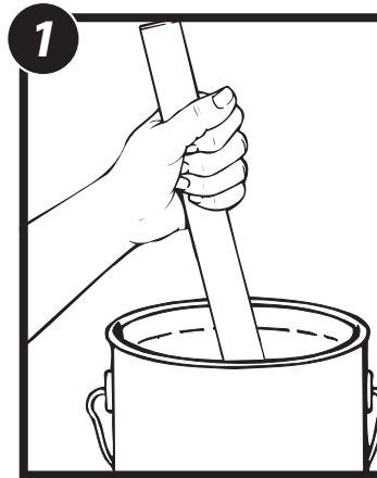
1. Stir the spraying material thoroughly.
