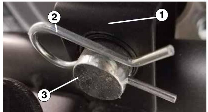
5. Install the hairpin cotter through the axle pin to lock it in place.
