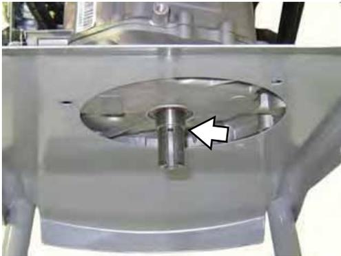
6. Slide the pump onto the crankshaft making sure the key lines with the keyway in the pump.
