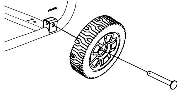
4. Install the wheel with axle pin through the axle bracket on the frame. The eye of the bolt should be facing toward the inside of the pressure.
