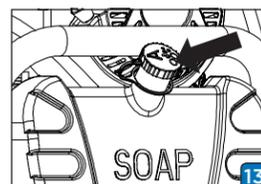
If you are using detergent on WPX2800/3100. Add detergent to soap tank. Only use detergent designed for pressure washer use.
